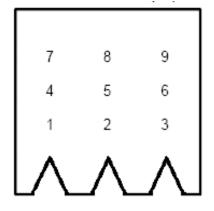
**Note:** To obtain local control using the internal potentiometer accessible at the top of the unit, jumper P2 pin 4 to pin 9.
