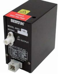
Spellman's Bertan brand of 605C modular high voltage power supplies offer well regulated, fixed polarity outputs up to 20kV, which operate off a +28Vdc input (+24Vdc optional). These fully enclosed modules are designed for bench top or OEM applications like spectrometers, detectors, imaging and electron beam usage.
